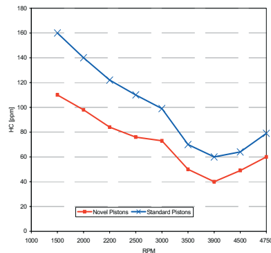
Fig. 14. Hydrocarbons emission (HC) for standard engine and engine with novel pistons versus engine speed at full load
